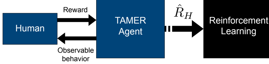
Figure 4.1: A conceptual diagram of sequential TAMER+RL. The human interacts directly with the TAMER agent. After training completes, the model of human reward, \hat{R}_H , is used by the RL algorithm along with MDP reward. Note that the task environment and MDP reward are not explicitly shown here; both the TAMER agent and the augmented RL agent interact with the environment, but only the RL agent receives MDP reward.
